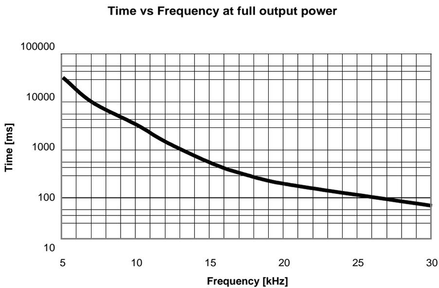
Figure 12: Duration of full output vs. frequency
