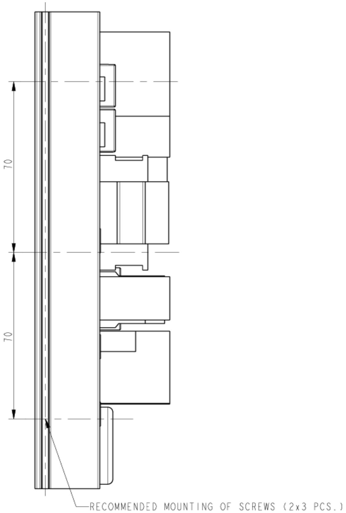
Figure 24: Physical dimensions for mounting slots in mm.
