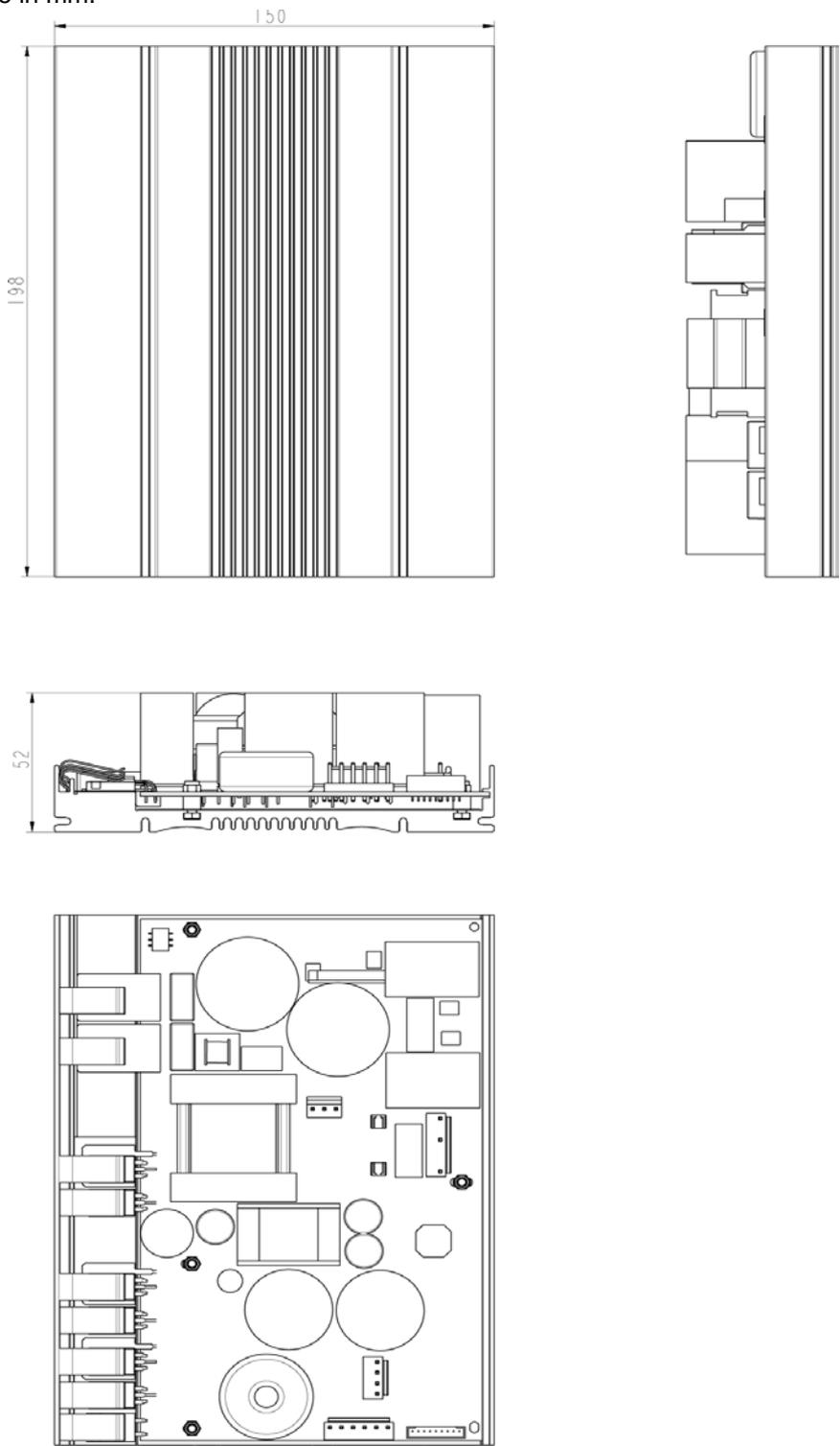
Figure 22: Physical dimensions in mm.
