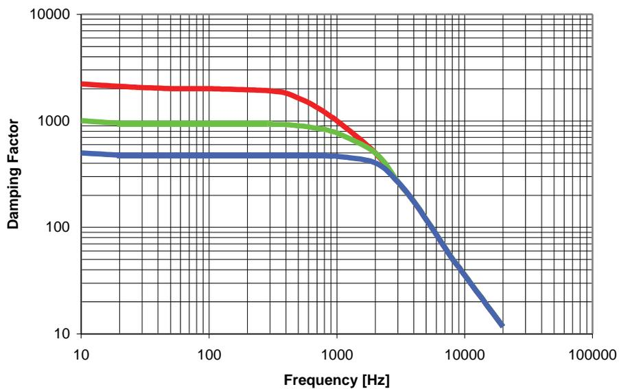
Figure 7: Damping factor vs. frequency 4Ω.
