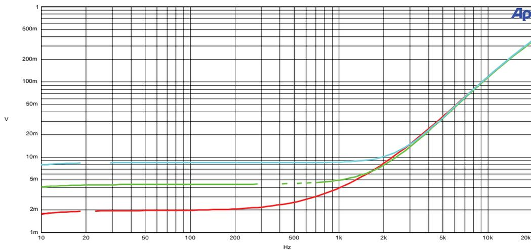
Figure 5: Measured voltage at output terminals while feeding 1A<sub>RMS</sub> into the output of the amplifier.
