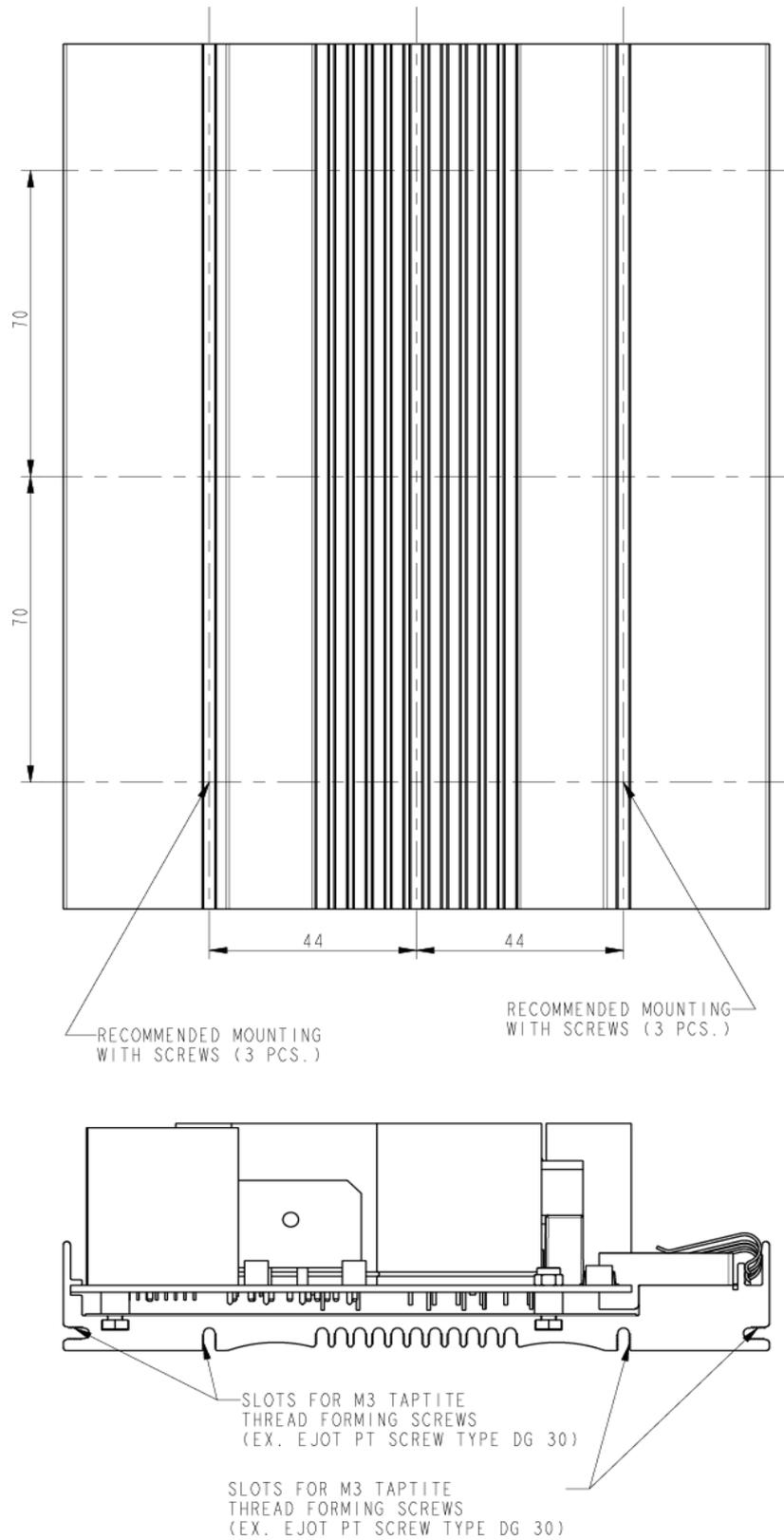
Figure 23: Physical dimensions for mounting slots in mm
