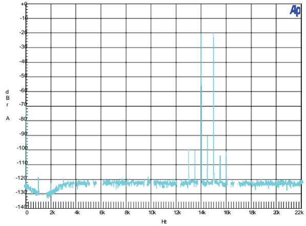
CCIF IMD analysis.  $R_L = 4\Omega$ ,  $P_O = 10\text{W}$ ,  $\text{IMD} = 0.00045\%$ .
