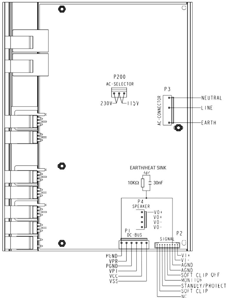
Figure 3: ICEpower500ASP connections
