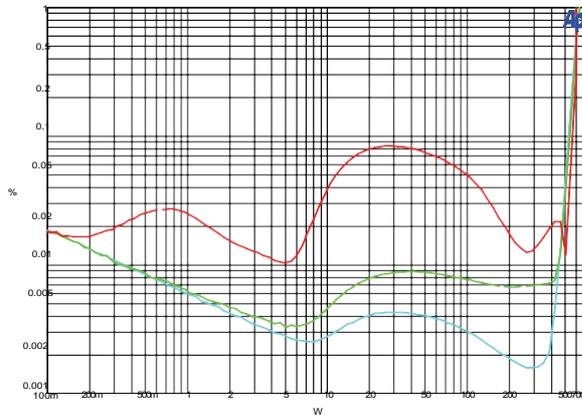
THD+N vs. output power at 100Hz, 1kHz and 6.67kHz <sup>4)</sup> (4Ω).
