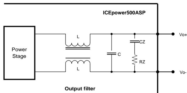
Figure 20: Output filter section with compensating Zobel network.
