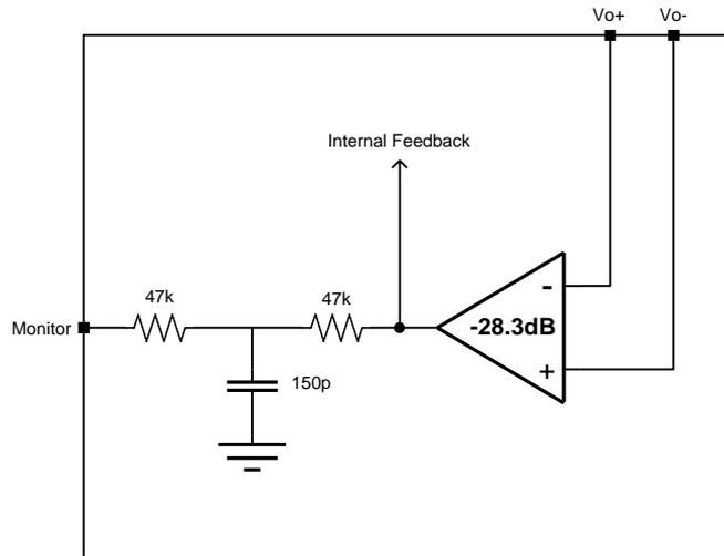
Figure 16: Internal circuitry of the monitor output.
