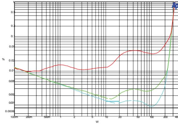
THD+N vs. output power at 100Hz, 1kHz and 6.67kHz <sup>4)</sup> (8Ω).
