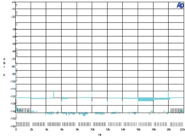
f = 5kHz. Po = 100mW. 4Ω loading.
