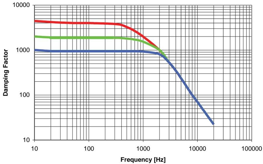
Figure 6: Damping factor vs. frequency 8Ω.
