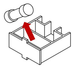
**Step 3:** Insert extra supplied EU fuse and place back the fuse holder into the IEC socket.
