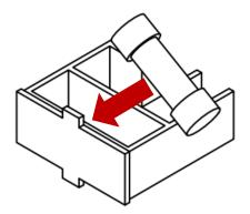
**Step 4:** Set the voltage selector switch in the 230 position. The amplifier is now set for 230V operation.
