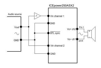
Figure 17: Wiring diagram for the BTL module
