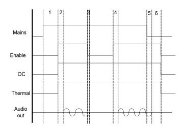
Figure 19: Timing – enable and mains
