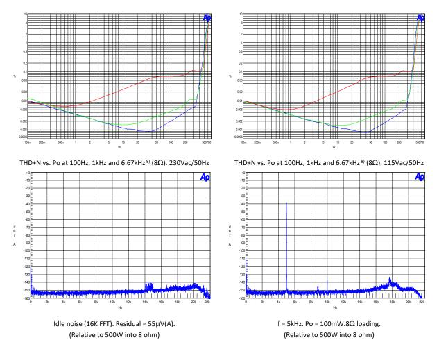
Figure 6: Total harmonic distortion & noise (BTL).
