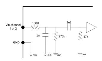
Figure 16: Single ended input buffer
