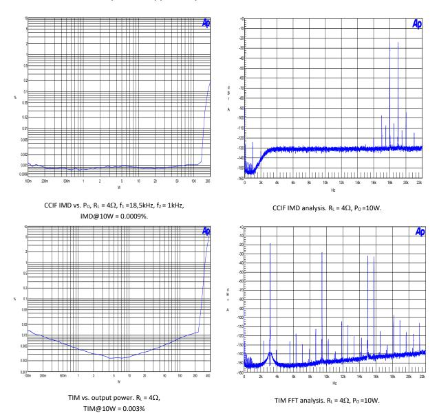
Figure 7: Intermodulation distortion (SE)
