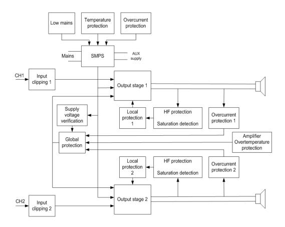
Figure 15: Protection schematic
