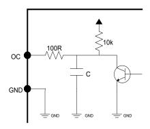
Figure 10: Over Current monitor pin interface.
