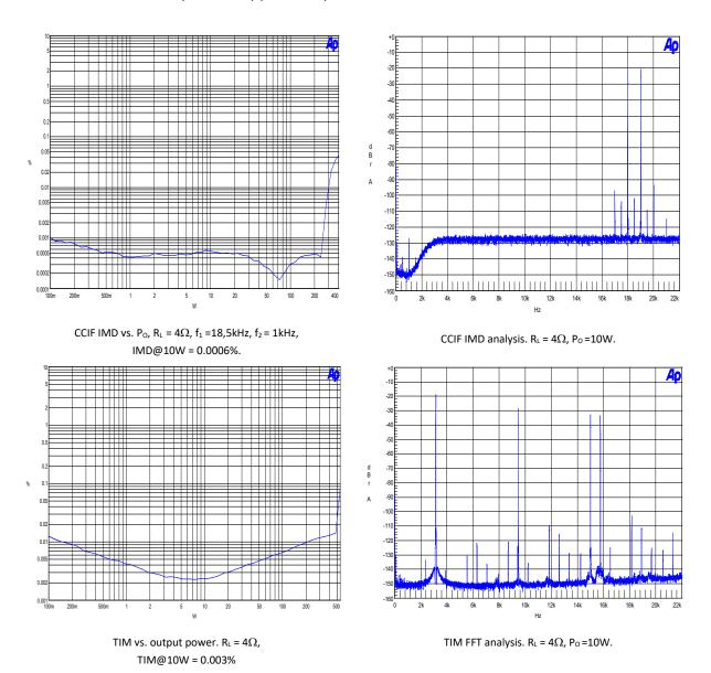
Figure 8: Intermodulation distortion (BTL)
