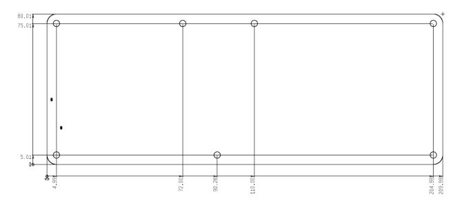
Figure 21: PCB drill pattern.
