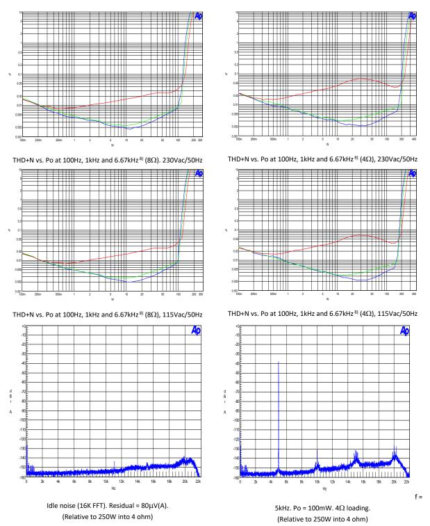
Figure 5: Total harmonic distortion & noise (SE).
