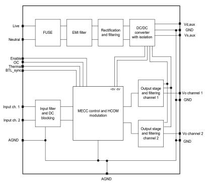
Figure 1: ICEpower250ASX2 block diagram
