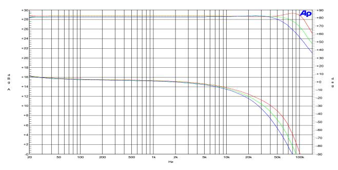
Figure 3: Frequency response in  $4\Omega$  (blue),  $8\Omega$  (green) and open load (red). Top – amplitude. Bottom – phase.
