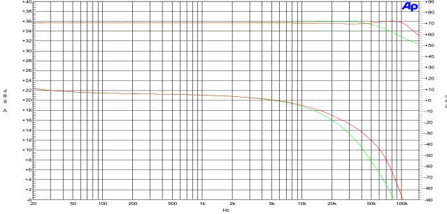
Figure 4: Frequency response in  $8\Omega$  (green) and open load (red). Top – amplitude. Bottom – phase.
