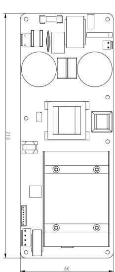
**Important!** A minimum clearance of 12 mm. around the module is required for safety and ventilation reasons.
