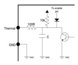
Figure 11: Thermal monitor pin interface.
