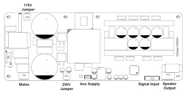
Figure 2: ICEpower250ASX2 connections
