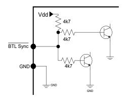
Figure 13: BTL sync pin interface.
