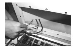
7. Seal all the cable holes with hot melt glue.
