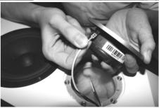
13. Mount the drivers to the cabinet and carefully tighten the screws.
