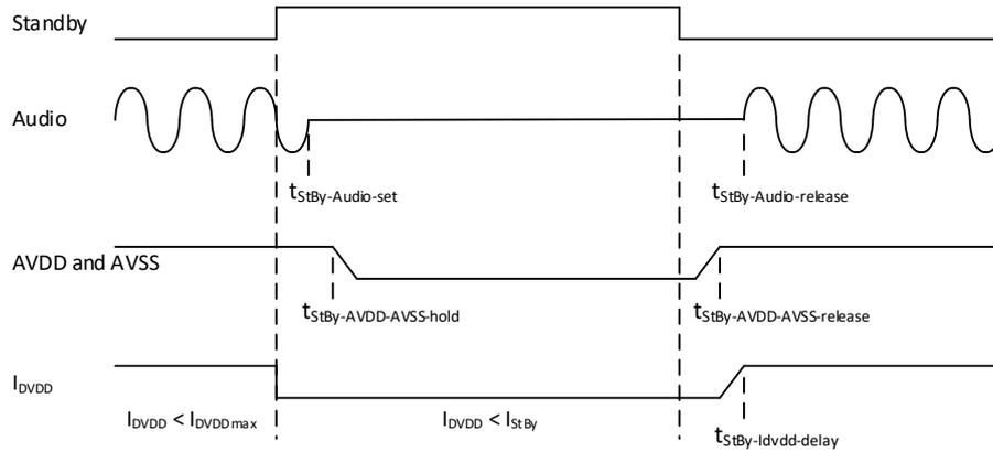
Figure 19: Standby timing on auxiliary supplies
