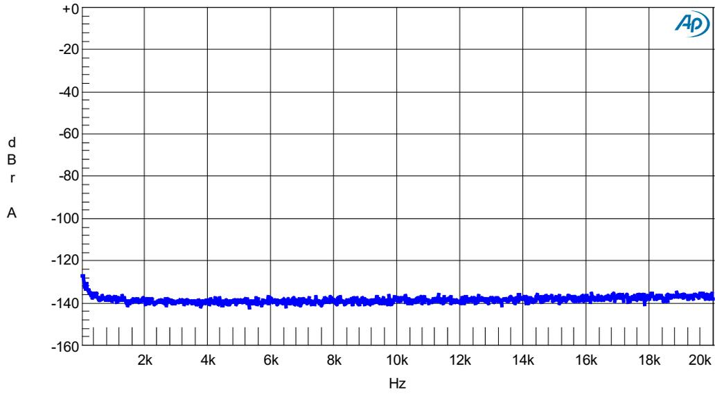
Figure 7: Idle noise (16kFFT) 0-20kHz @ 0dB = 100 W/4 Ω
