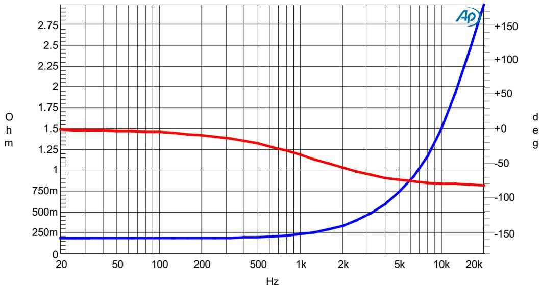
Figure 10: Output impedance vs frequency 20-20kHz (blue), phase (red)
