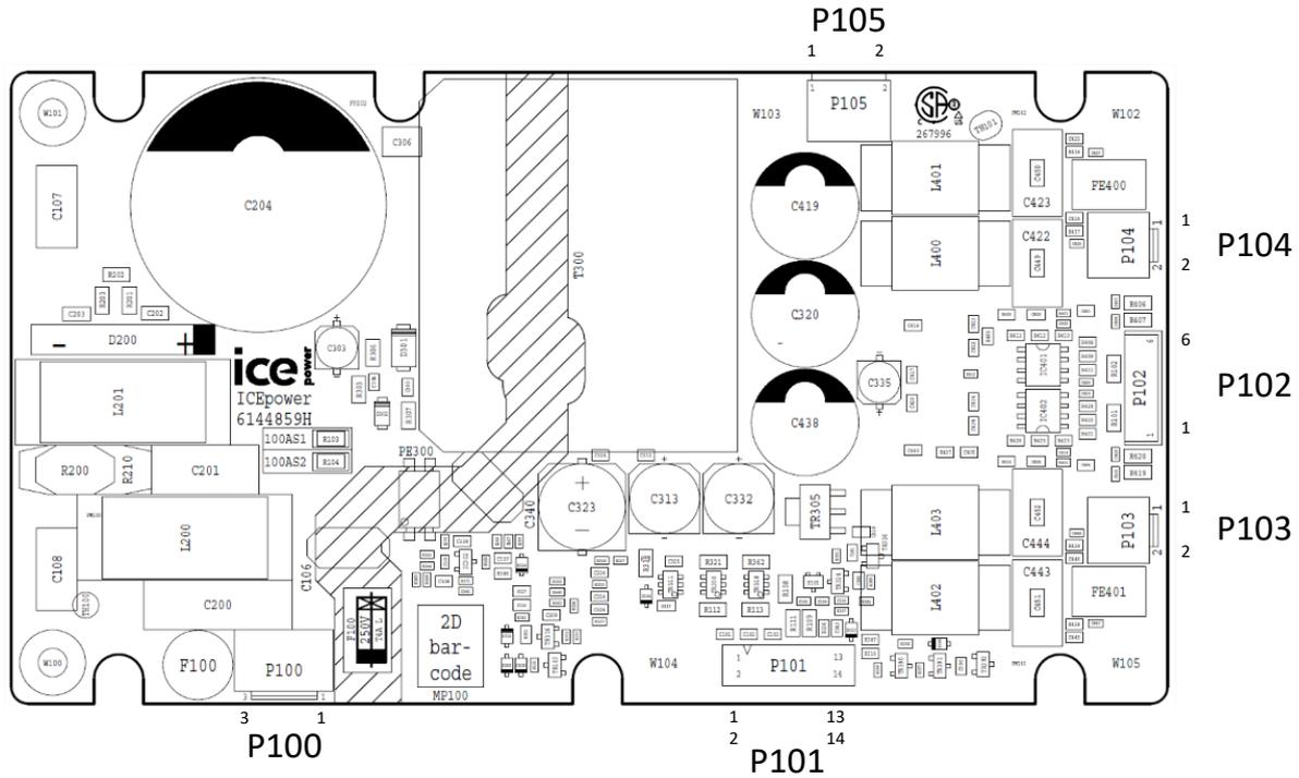
Figure 2: ICEpower100AS1/2 connector overview
