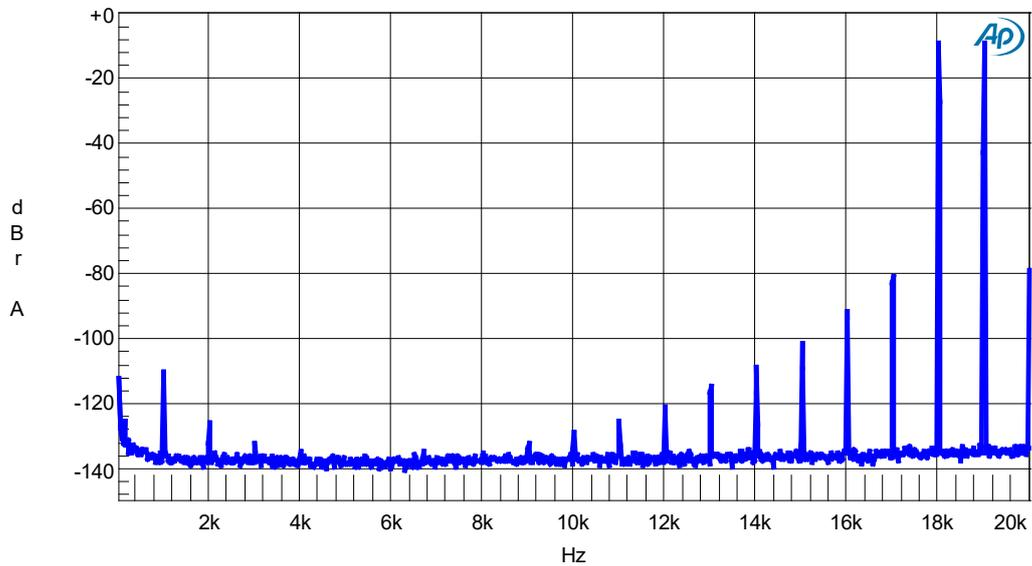
Figure 8: Intermodulation (16kFFT) 0-20kHz @ 0dB = 100 W/4 Ω
