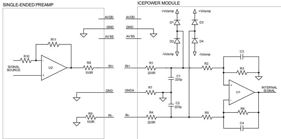
Figure 24: Analog input interface schematics
