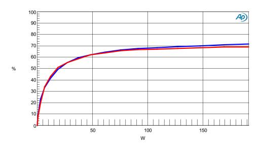
Figure 12: Power efficiency vs. output power, 230  $V_{ac}$  / 50 Hz (blue), 120  $V_{ac}$  / 60 Hz (red)
