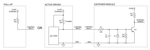
Figure 21: Control input interface schematics
