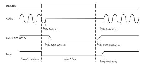
Figure 15: Standby timing on auxiliary supplies
