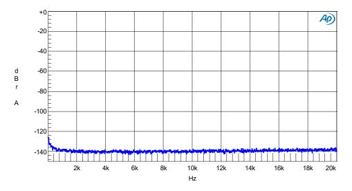
Figure 7: Idle noise spectrum, 0 – 20 kHz @ 0dB = 200 W / 4  $\Omega$
