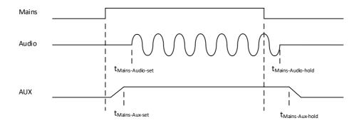
Figure 14: Power up timing
