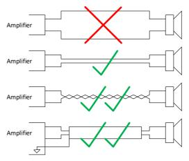
Figure 24: Speaker wire routing
