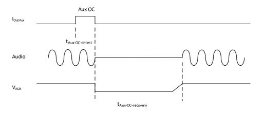
Figure 18: Auxiliary supply overcurrent timing
