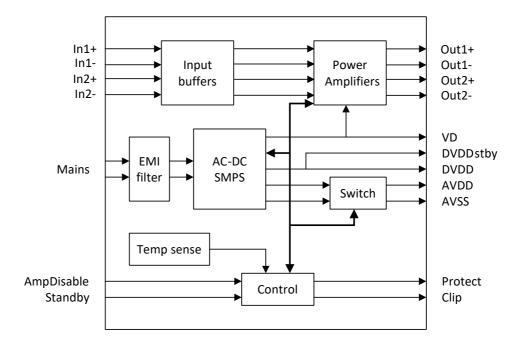
Figure 1: ICEpower200AS2 block diagram
