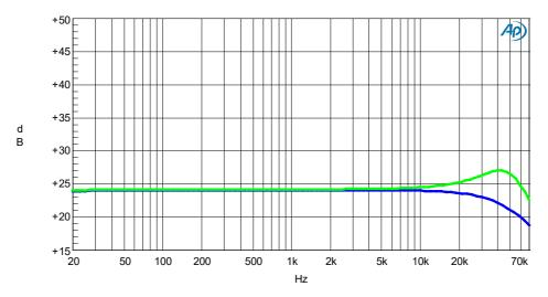
Figure 4: Amplitude vs frequency @  $R_L=4~\Omega$  (blue) and  $R_L=8~\Omega$  (green). For more details see ICEpower100AS1/2 200AS1/2 Application Note.
