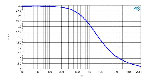
Figure 10: Damping factor vs. frequency, 20 Hz – 20 kHz, 4  $\Omega$  (blue)
