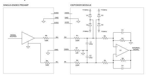
Figure 20: Analog input interface schematics
