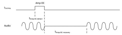
Figure 17: Speaker output overcurrent timing
