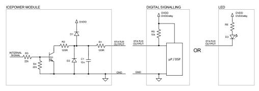
Figure 22: Status output interface schematics
