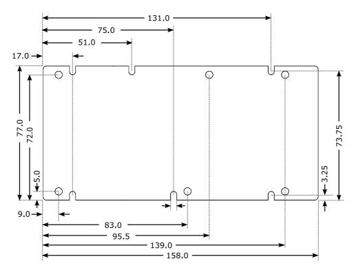
Figure 3: ICEpower200AS2 baseplate mechanical dimensions in mm seen from top side  $\frac{1}{2}$
