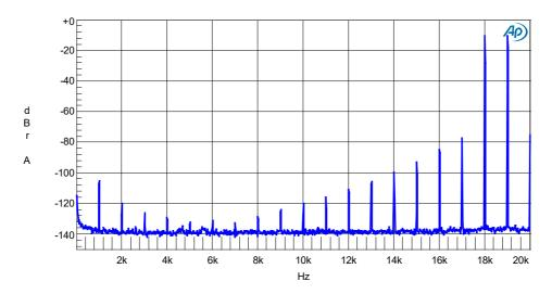
Figure 8: Dual tone intermodulation spectrum, 0 – 20 kHz @ 0 dB = 200 W / 4  $\Omega$
